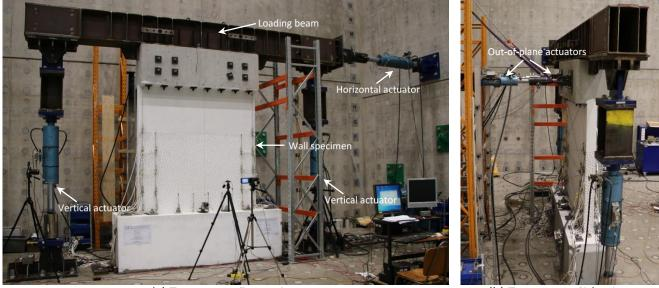
(a) Test setup: Front view
