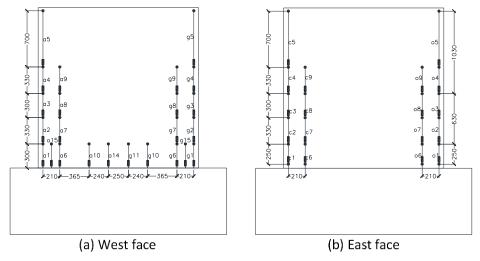
Figure 3: Instrumentation: Linear potentiometer provided on wall specimens
