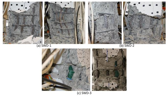
Figure 7: Reinforcement buckling observed during the tests conducted in this study
