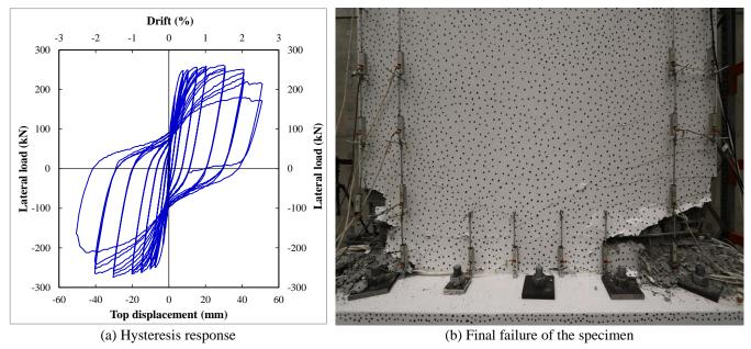
Figure 4: Hysteresis response of wall specimen SWD-1
