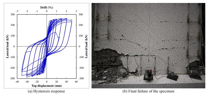
Figure 6: Hysteresis response of wall specimen SWD-3
