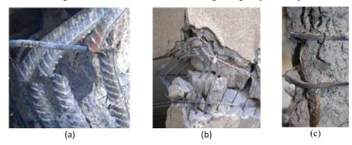
Figure 1: Damage observed in RC walls during the past earthquakes and wall tests (a) Fracture [1], (b) Buckling [1], (c) Buckling [2]
