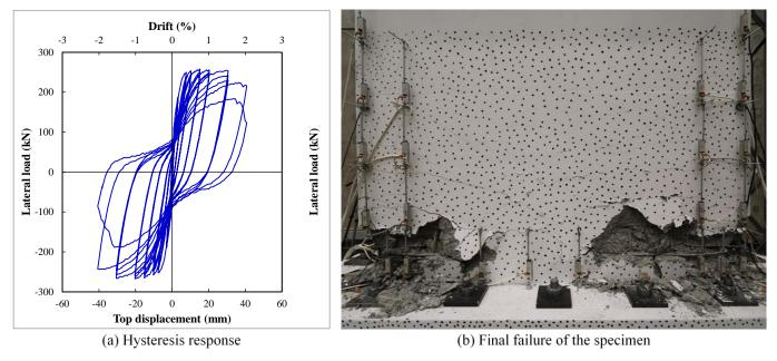
Figure 5: Hysteresis response of wall specimen SWD-2
